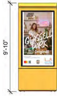
Wave Urban Panel Plan & Elevation Scale: 3/16" = 1'-0"
