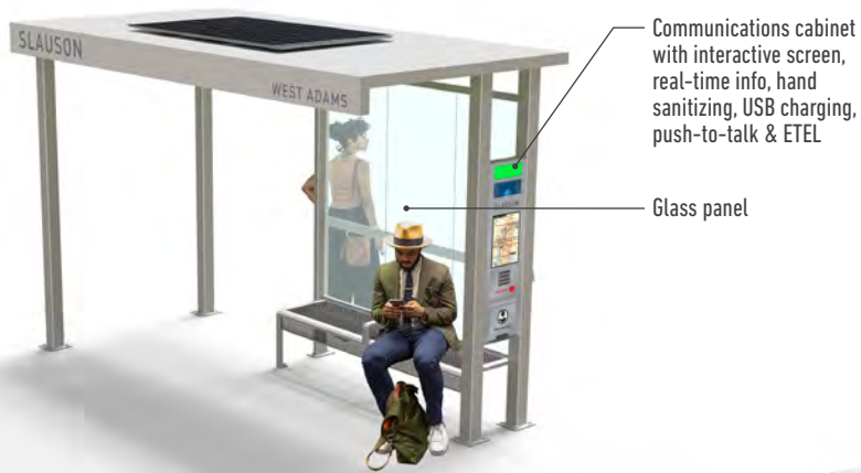
SHELTER WITH COMMUNICATIONS CABINET
